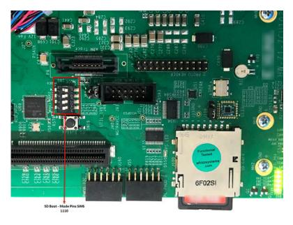
This graphic shows the configuration settings for the Xilinx Zynq UltraScale+  $^{\rm TM}$  MPSoC ZCU102 FPGA development board.
